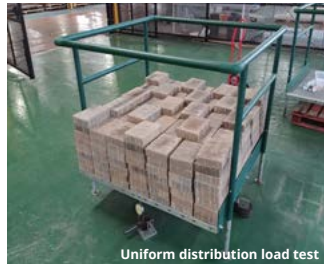
Uniform distribution load test
